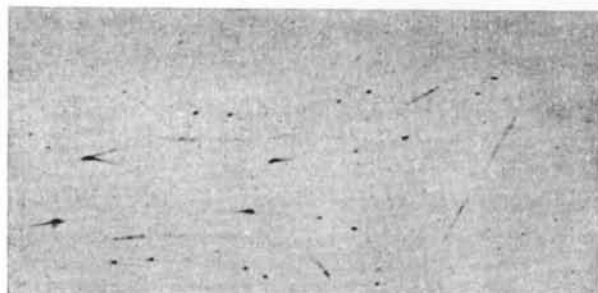
Fig. 1. First-layer equi-inclination Weissenberg photograph, b -axis rotation.
